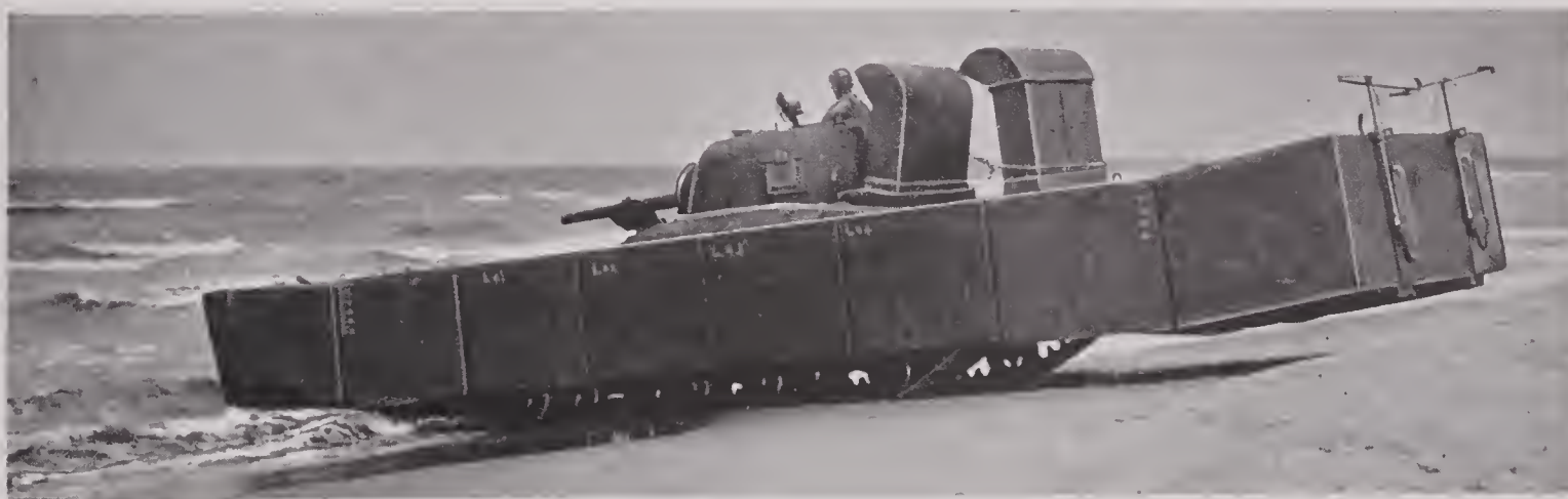
FIGURE 1. M-4 A1 medium tank equipped with Ritchie T-6 flotation device.
